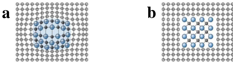
Fig. 14. Two types of particles depending on crystallographic correlation of matrix and precipitation: a) coherent - with relationship between the crystallographic planes, b) incoherent - no relationship with the crystallographic planes.
