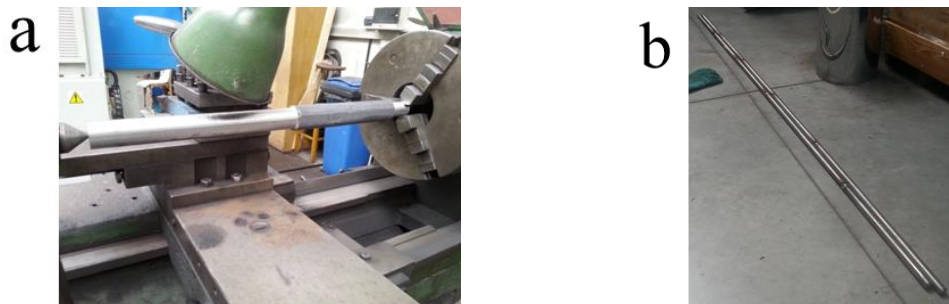
Fig. 38. The next steps of machining steel with a modified chemical composition: a) machining process of material after forging on a rod with a diameter of Ø30 mm, b) connected rods made of experimental melts, consisting of 5 different materials.
