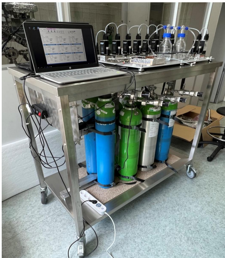
Fig. 8.4. SPV gas sensor device at the Department of Cybernetics, Nanotechnology and Data Processing, Silesian University of Technology, Gliwice, Poland.
