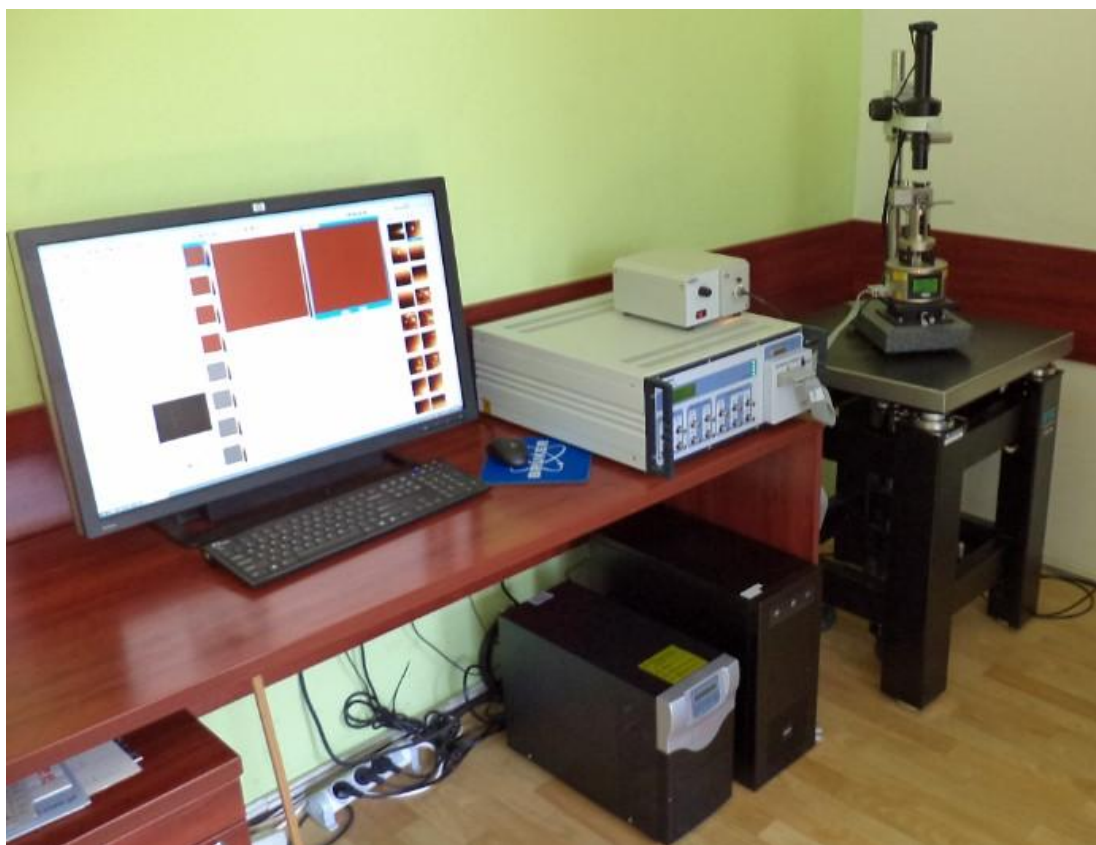
Fig. 5.2. Atomic Force Microscope at Department of Cybernetics, Nanotechnology and Data Processing, Silesian University of Technology, Gliwice, Poland.
