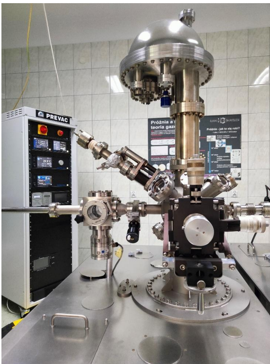
Fig. 5.5. X-ray Photoelectron Spectrometer (XPS) at the Department of Cybernetics, Nanotechnology and Data Processing, Silesian University of Technology, Gliwice, Poland.
