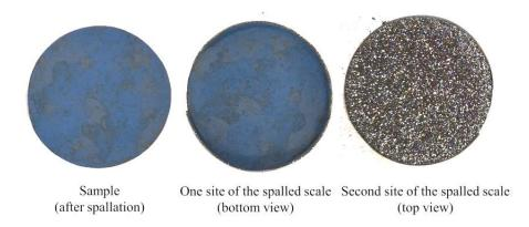
Figure 5.6: Macrographs showing the ORE sample after severe oxide spallation during longterm cyclic oxidation at 900 °C.
