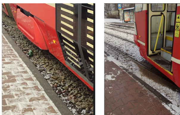
Fig. 5.5. Example of the architecture barrier: a long distance between tram and sidewalk makes this stop not adapted to people with special needs
