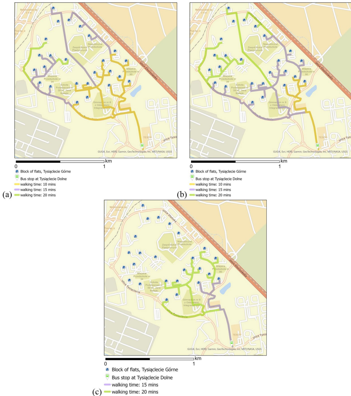
Fig. 5.10. The distance that can be reached by pedestrian depends on the speed (a) 6 km/h; (b) 5 km/h, and (c) 3 km/h, respectively), if they move from Tysiąclecie Dolne to Tysiąclecie Górne estate on foot, due to a lack of connection between two parts of the estate
