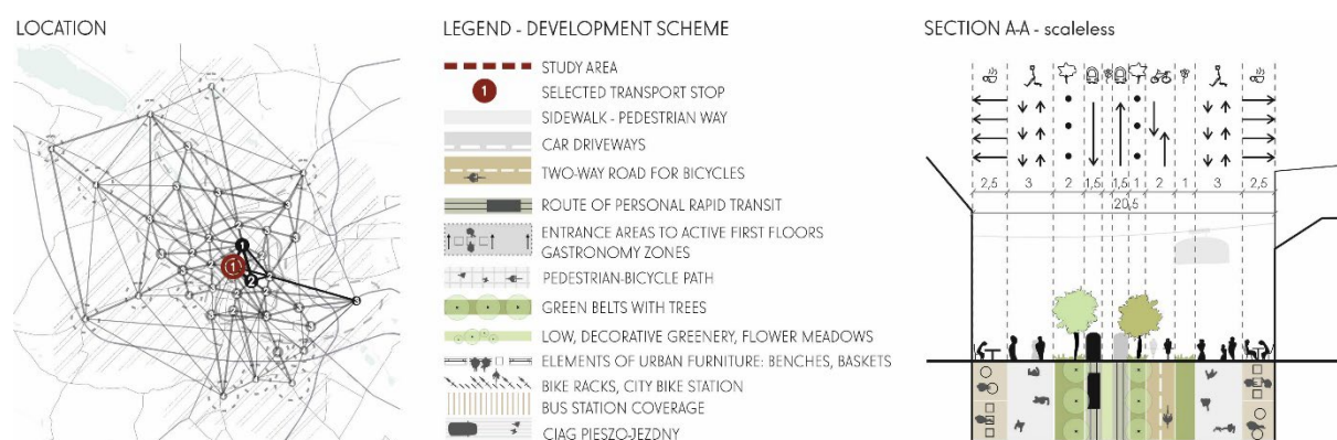
Fig. 4.13. Legend and site section for A schematic concept of the center zone development
