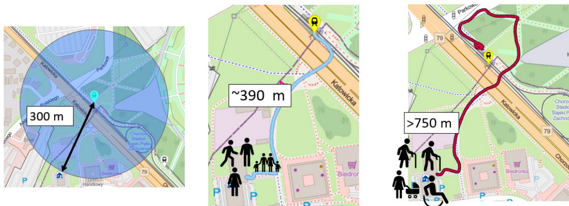
Fig. 5.3. Comparison of the distance to go as a linear and along network that must be passed by people (PNP and PPM) and existing architectural barriers
