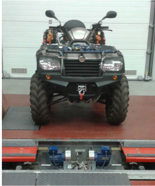
Fig. 8.5. Experimental off-road vehicle and laboratory setup for suspension diagnostics
