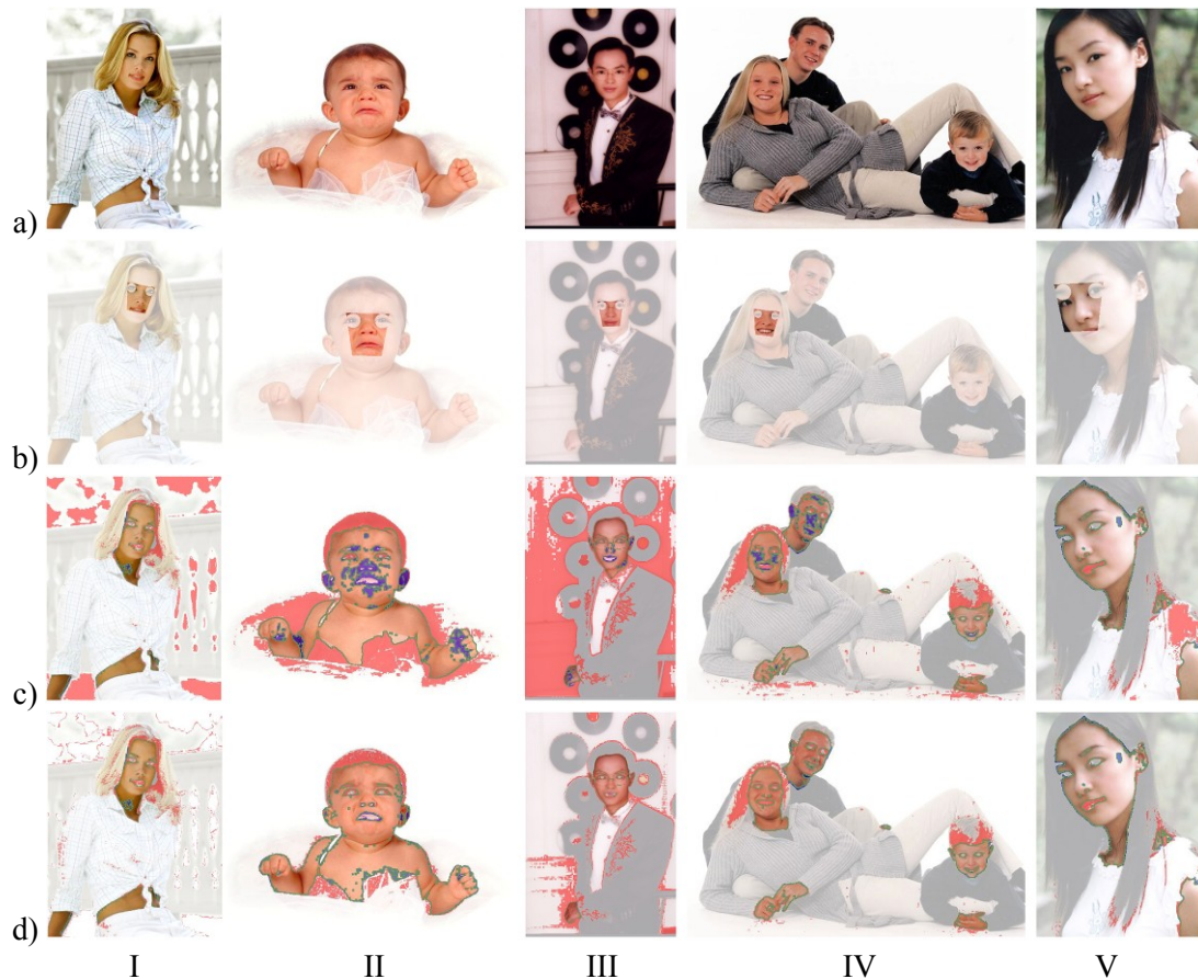
Fig. 4. Skin segmentation results: a) input images, b) facial regions, c) segmentation results obtained using Cheddad's method and d) using proposed adaptation
