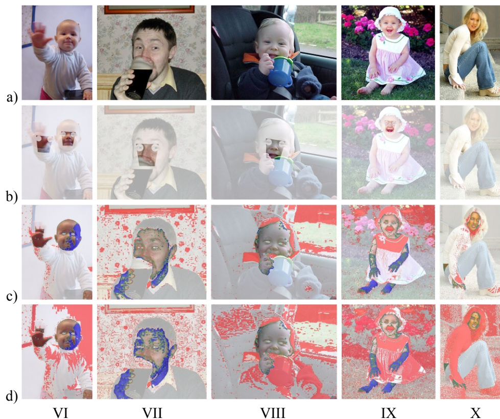
Fig. 5. Skin segmentation results: a) input images, b) facial regions, c) segmentation results obtained using Cheddad's method and d) using proposed adaptation
