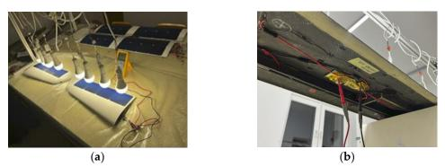
**Figure 8.7.** Verification tests on the test stands: (a) Irradiation of the solar cells placed in the winglets with 200 watts led bulbs; (b) Single solar cell test.
