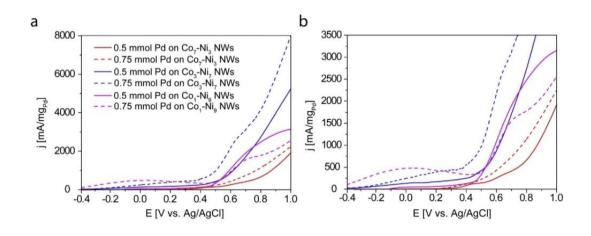
Fig. 10. (a) Comparison of the cyclic voltammograms of electrocatalysts in the form of cobalt-nickel nanowires with different Co:Ni ratios decorated by Pd in argon-saturated 1.0 M NaOH + 0.5 M  $CH_3CH_2OH$  solution at a scan rate of 20 mV/s; (b) plot showing an enlargement of the data between 0 and 3500 mA/mg<sub>Pd</sub>. Reproduced and modified with permission from <sup>10</sup>. Copyright (2022) Elsevier.
