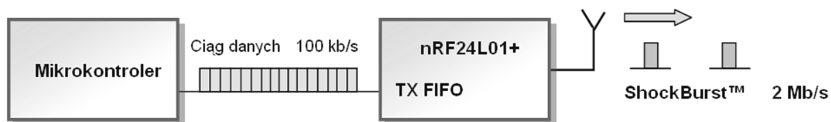
Rys. 1. Technologia ShockBurst TM
