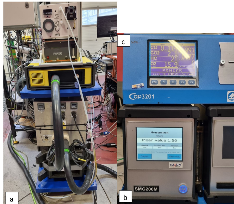
FIGURE 2.1: Emissions measurement equipment: a) FTIR, b) SMG200M PM device, and c) Capelec gas analyzer.
