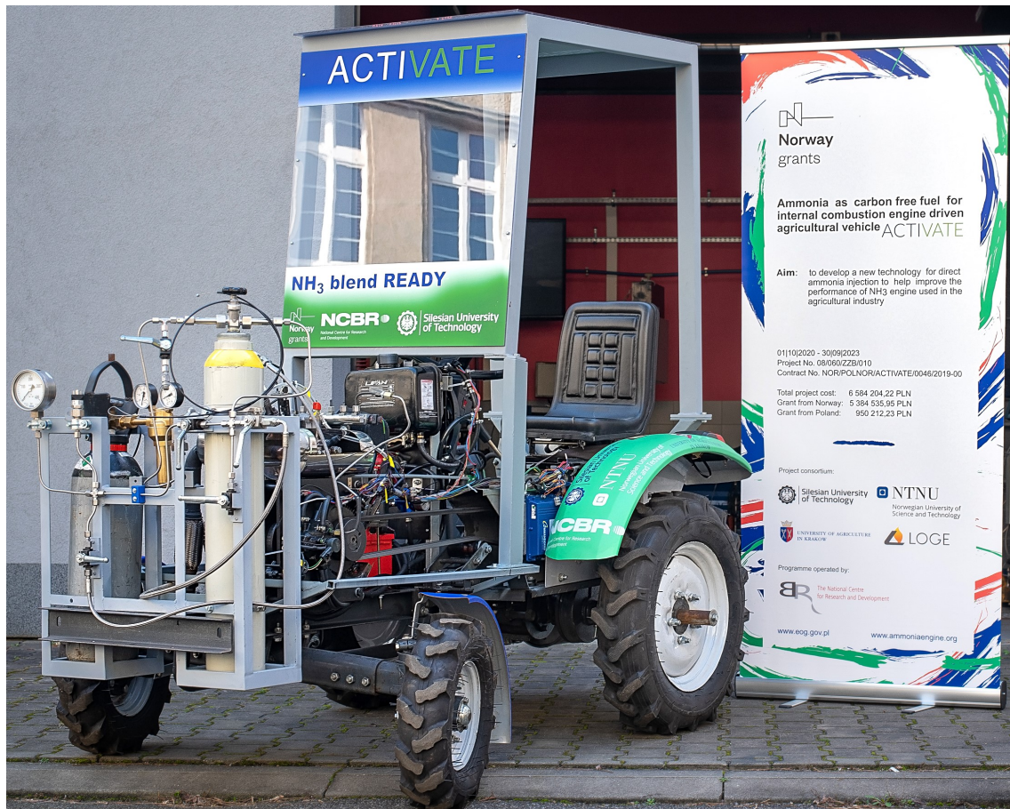
FIGURE 6.1: Liquid ammonia-biodiesel fueled prototype agriculture tractor
