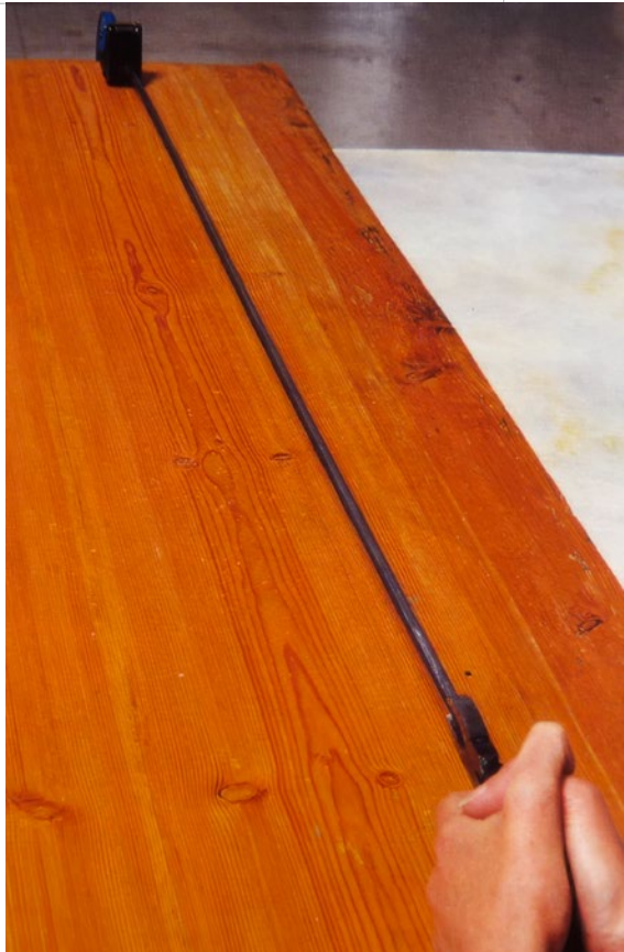
Fig. 68. Lead profile stretching with a clamp on the table
