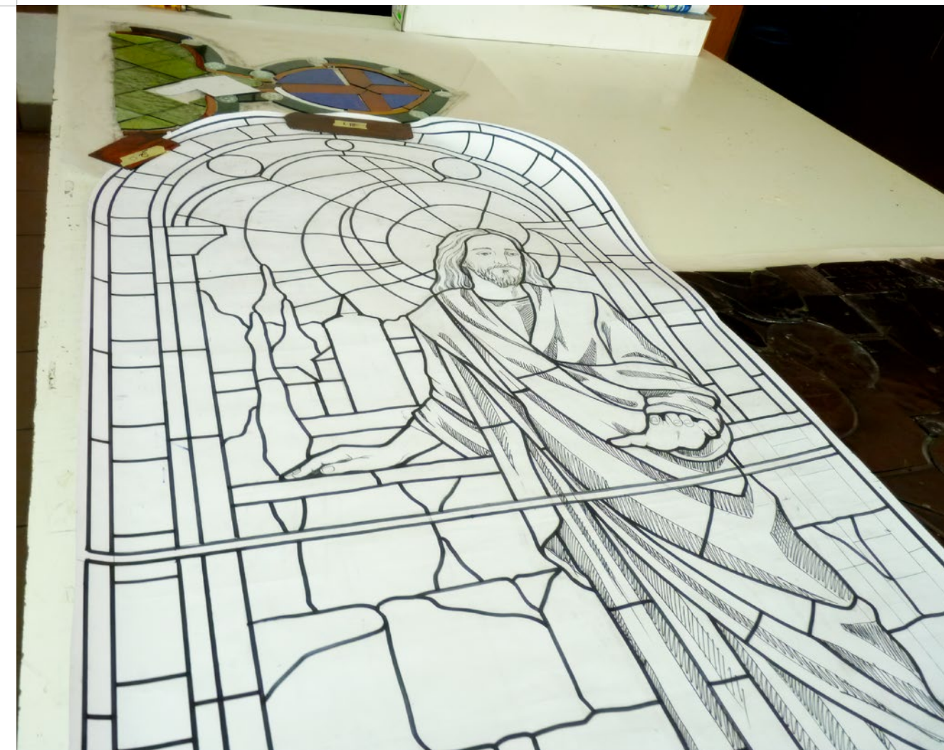
Fig. 62. Stained glass window mock-up drawing at a scale of 1:1; preparation for glass cutting
