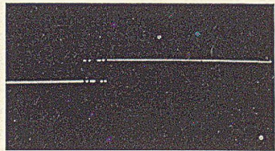
Fig. 21—Typical chatter on closure of contacts.
