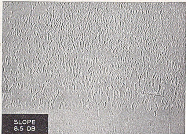
Fig. 16—Three pictures showing the appearance of the error signal when using 'slope' prediction.
