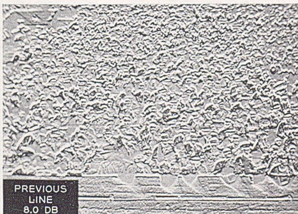
Fig. 17—Three pictures showing the appearance of the error signal when using "previous line" prediction. Note the absence of vertical contours.
