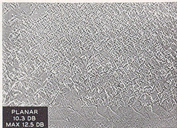
Fig. 18—Three pictures showing the appearance of the error signal when using “planar” prediction. Note the absence of horizontal and vertical contours.
