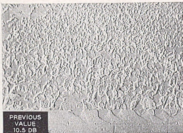
Fig. 15—Three pictures showing the appearance of the error signal when using "previous value" prediction. Note the absence of horizontal contours.
