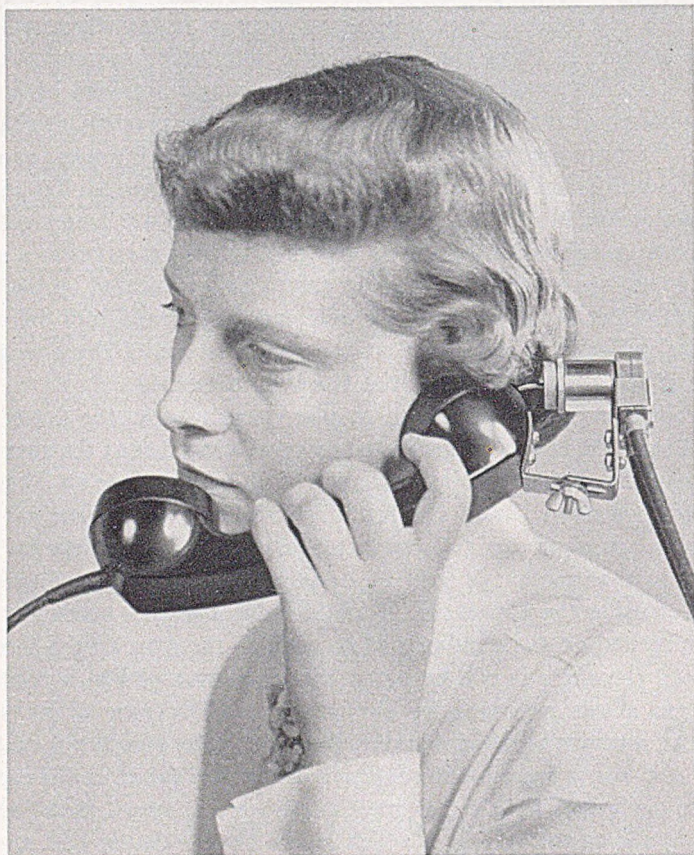
Fig. 5—Method of measuring receiver response on a human ear, using a search tube microphone.
