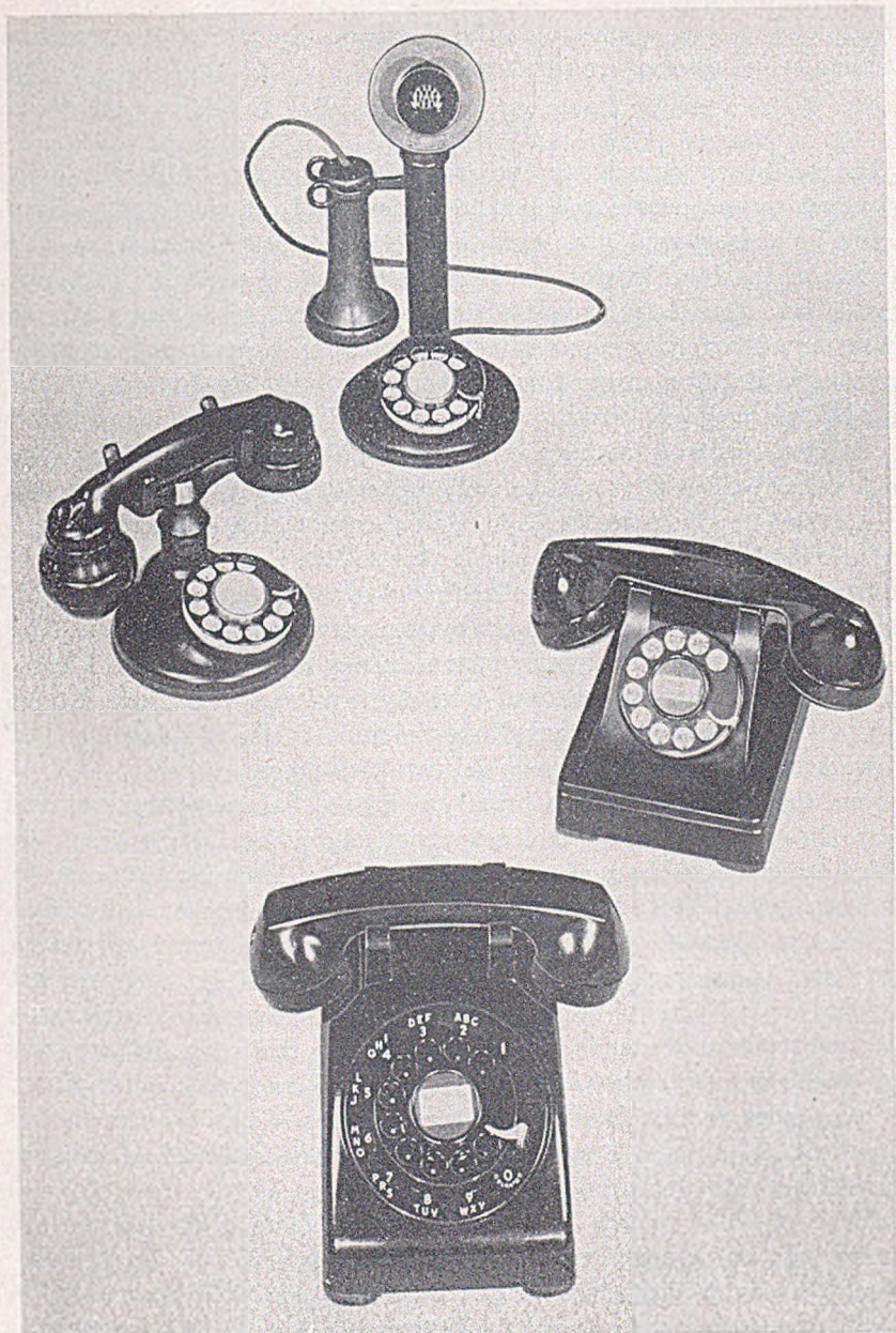
FIG. 3—The telephone deskstand of 1919, at top; the handset of 1927, left center; the combined set of 1937, right center; and the 500-type set of 1950, bottom.
