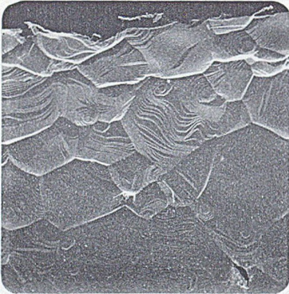
Fig. 9—Aluminum replica ( \bar{l}_e = 180 \text{ \AA} , \theta_a = 30^\circ ) showing granularity due to recrystallization. Local curling of replica has resulted in "negative shadows" in upper left region of stereogram. Resolution about 100 \text{ \AA} .
