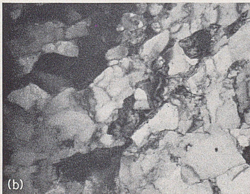
Fig. 12—Effect of temperature at which recovery proceeds on domain size in high purity aluminum.
