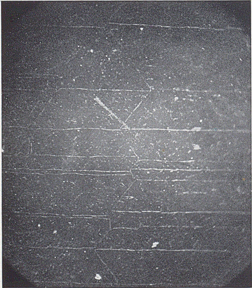
Fig. 13—Photograph of domains in a single nickel crystal (after Williams). Field of view, 0.5 mm.
