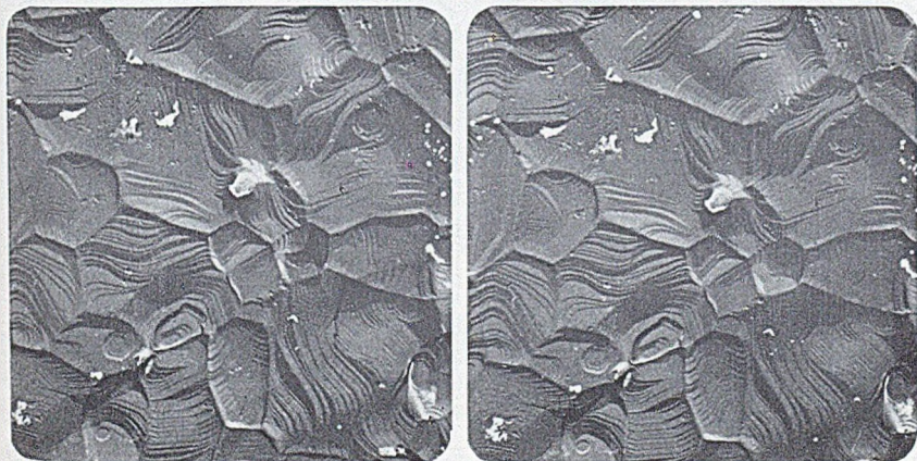
Fig. 10—Gold-manganin replica ( t_e = 150\text{\AA} , \theta_a = 20^\circ ). Resolution about 100\text{\AA} . Replica is much thicker than optimum. A film in the shadow, clearly evident in the original micrograph, does not show except for two whitish areas where it has torn and curled.
