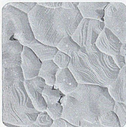
Fig. 7—Chromium replica ( i_c = 100\text{\AA} , \theta_a = 30^\circ ) of surface of a thermistor flake. Resolution about 50\text{\AA} . Granularity is due to plastic mold.
