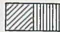
Fig. 3. „Bicellophane.“ The principal sections of the two adjacent pieces of cellophane make an angle of 45^\circ
