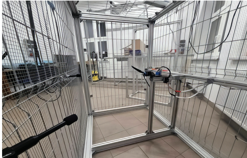
To test different types of propellers, the students built a station for measuring draft and noise levels in the form of a cage.
