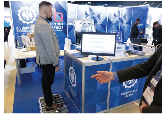
A device for measuring the distribution of foot pressure on the ground and the torque of forces rotating the lower limb.
