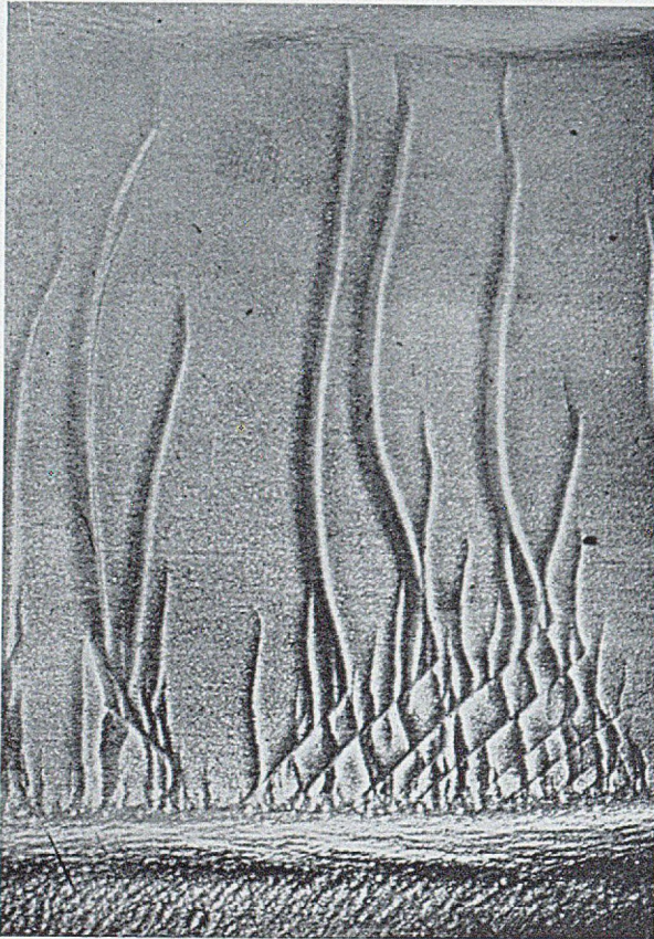
FIG. D.—Stretcher-Strain Markings on a Steel Pressing. \times 1 . (Hundy.)
