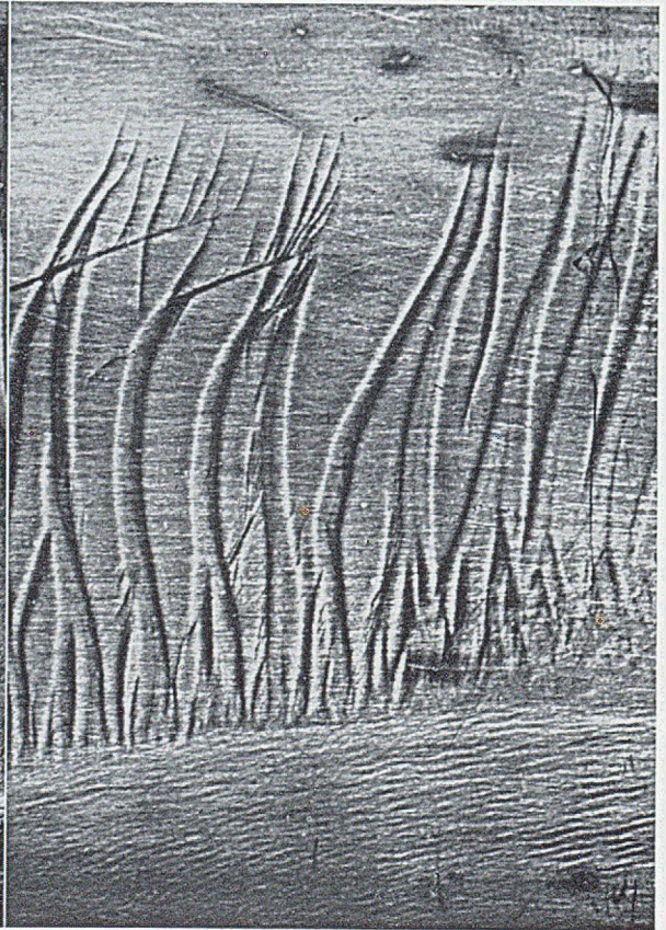
FIG. E.—Stretcher-Strain Markings on an Aluminium-Magnesium Alloy Pressing. \times 1 . (Hundy.)
