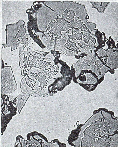
FIG. B.—Aluminium-6.37% Chromium Alloy, Chill-Cast and Annealed. \times 750 . ( Dudzinski's reply. )
