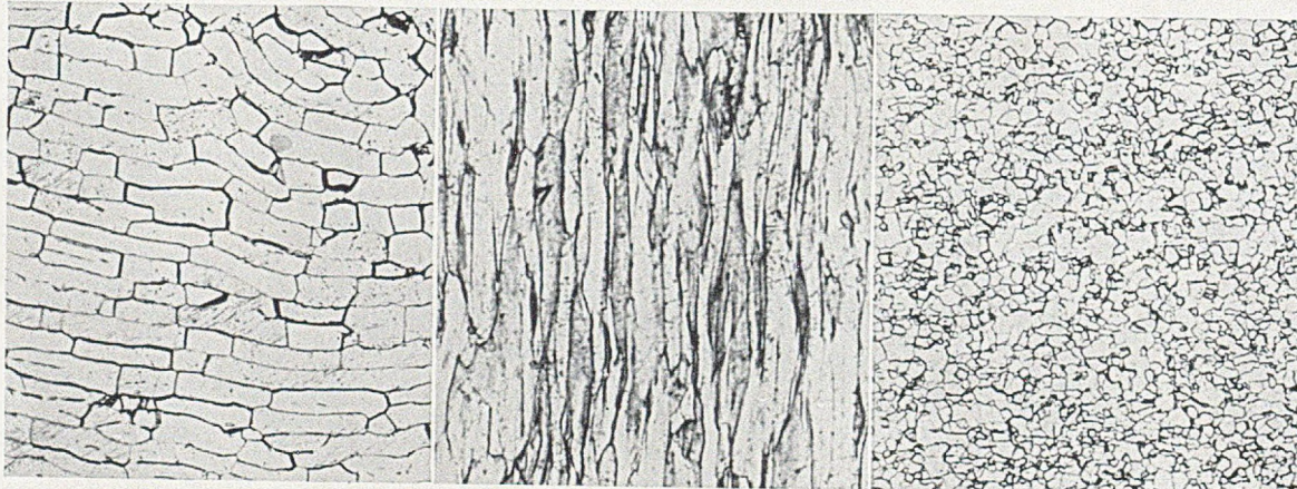
FIG. 11.—3 at.-% Oxygen Alloy Swaged at 900^{\circ} – 1000^{\circ} C., Heated at 1000^{\circ} C. for 5 Hr., and Cooled at 5^{\circ} C./min. \times 100 .
