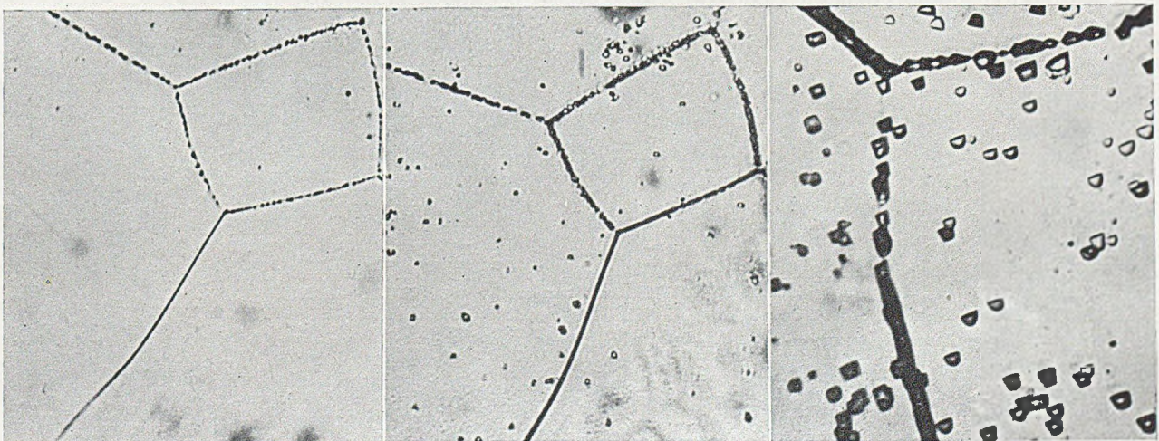
FIG. 6.—Grain-Boundary in Al-7% Mg Alloy Aged for 6 Hr. at 200° C. Etched for 10 sec. in Keller's Reagent. \times 1500 .
