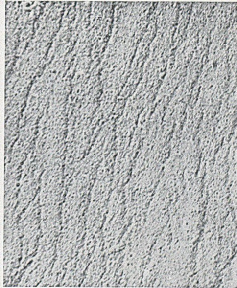
FIG. 5 (b).—Part of the Lamellar Structure of One of the Slip Bands Shown in Fig. 5 (a). Aluminium oxide replica shadowed with gold-palladium. \times 25,000 .
