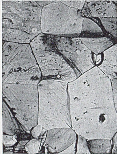
Typical Fields of Specimen Strained 3.07% in 66 Hr. at 1420 lb./in.². FIG. 2.—Etched in Ammonium Sulphide Solution. × 100.
