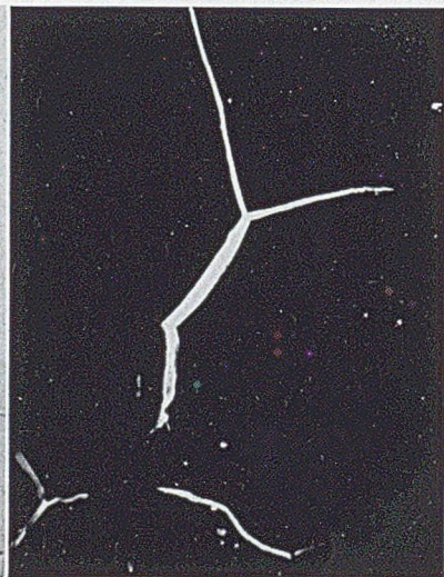
Appearance of "Thickened" Grain Boundaries Such As Shown at C in Fig. 7. FIG. 8.—Normal Illumination. × 500.
