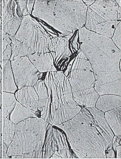
Typical Fields of Specimens Strained Approximately 0.2%. × 50. FIG. 4.—In 6 Hr. at 1300 lb./in.².
