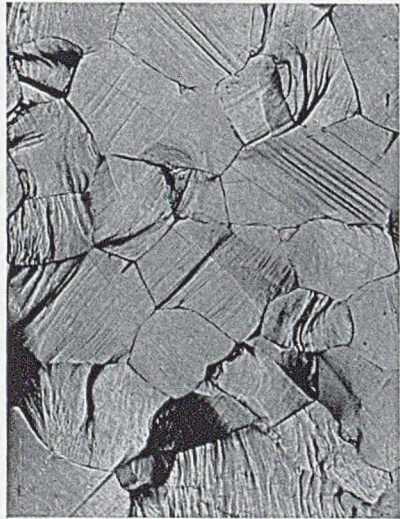
Specimen in Fig. 4 Further Strained to 1.4% in 71 Hr. at 1300 lb./in.². FIG. 6.—× 75.
