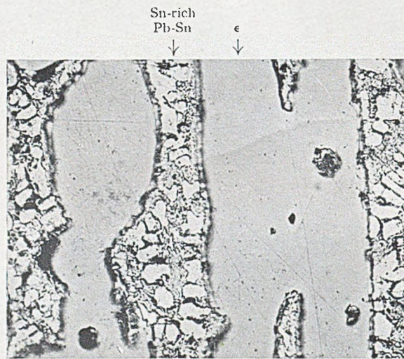
FIG. 27 (b).—Copper-Tin-Lead Alloy. Annealed 7 days at 400° C. \times 150 .
