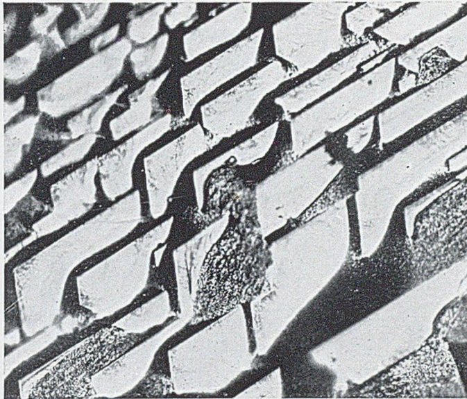
FIG. 18.—Appearance of Copper Grain Face after Immersion in Lead Saturated with Copper and Very Slow Cooling to Precipitate Primary Copper. Showing development of preferred planes and "liquid" retained in grooves of structure. \times 400 .
