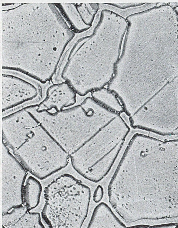
FIG. 16.—Dewetted Copper Surface Showing Attack at Grain Boundaries. Copper immersed in lead at 600° C. for 2 hr. \times 400 .
