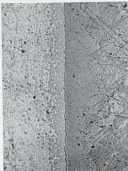
FIG. 23 (b).—As (a), but Immersed in Tin Containing 0.1% Nickel. × 500.
