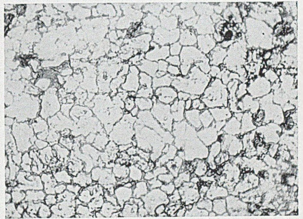
(b) Outer zone. Grain-boundary penetration is evident.
