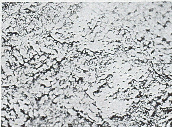
FIG. 20.—Copper Surface Immersed for 10 sec. at 400^{\circ}\text{C} . in Lead Containing 0.05% Tin, Showing Cubic Etch-pits on the Least Attacked Grains. \times 750 .
