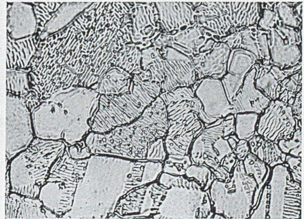
FIG. 21.—Copper Surface Immersed for 15 min. at 500^{\circ}\text{C} . in Lead Containing 2.5% Silver, Showing Form of Etching. \times 500 .
