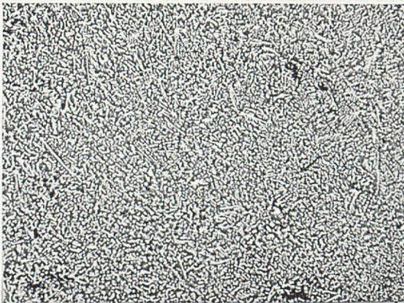
FIG. 13.—Small Dendrites in Interior of Al-20% Cu-0.04% B Alloy, Solidified under Centrifugal Force. Etched in 0.5% HF. \times 15 .
