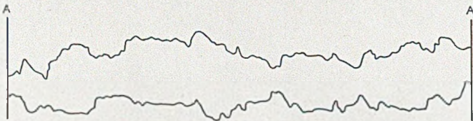
FIGS. 5-10.—Strain Markings Obtained by the Progressive Stretching of an Aluminium-Magnesium Alloy Sheet of 0.025 mm. Grain-Size, with Talysurf Traces of Upper and Lower Surfaces from A to A' .
