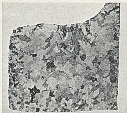
FIG. 5.—Al-5% Cu-0.04% B Alloy, Centrifuged for 15 min. at 655^\circ C . \times 3 .
