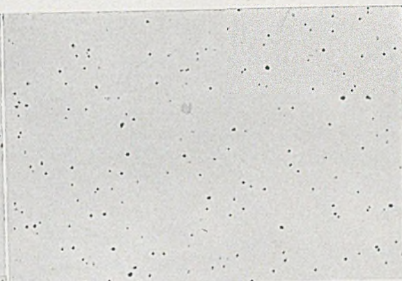
FIG. 3.—Section of Same Metal after Remelting and Repeated Fluxing. P = 0.1%. Unetched. \times 50 .
