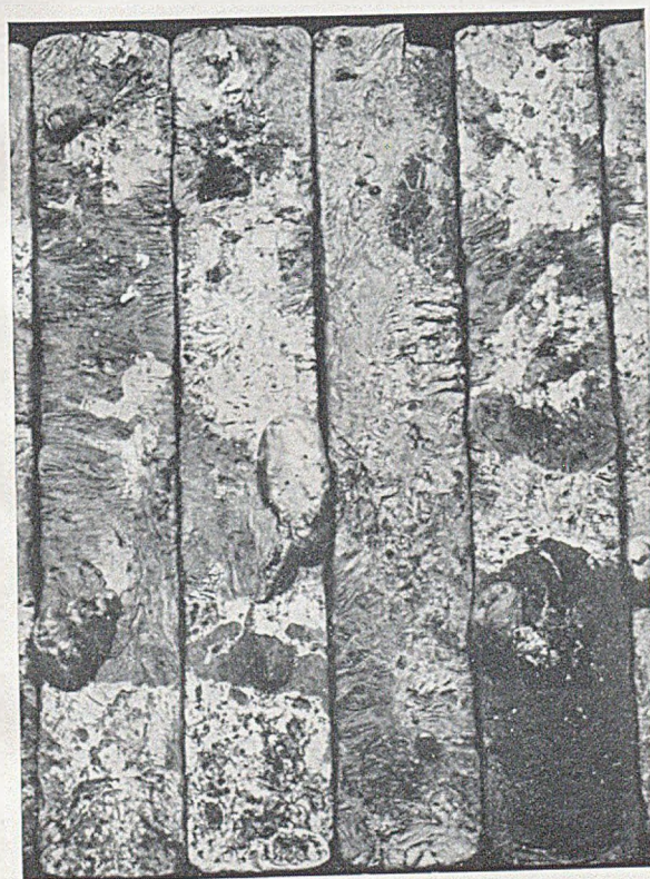
FIG. 6.—Ingot Poured at 750° C. from a Melt of Magnesium Saturated with Phosphorus, Showing Extensive Areas of Oxidation and General "Gassy" Appearance. \times 4 .
