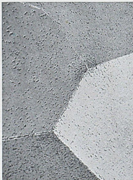
FIG. 6.—Pb-0.85% Sb Alloy Solution-Treated at 300° C., Water-Quenched and Aged 120 Hr. at 50° C. Slight continuous precipitation within grains; mainly in form of widely distributed needles. \times 300 .
