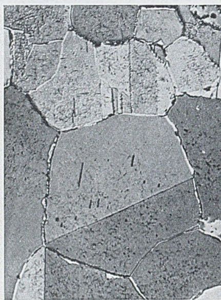
FIG. 5.—Pb-0.85% Sb Alloy Air-Cooled after Extrusion at 160° C. and Aged at 20° C. for 12,000 Hr. Continuous precipitation within grains. \times 300 .
