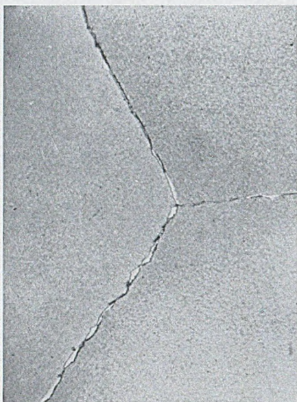
FIG. 4.—Pb-0.85% Sb Alloy Air-Cooled after Extrusion at 300° C. Slight discontinuous precipitation at grain boundaries, although no continuous precipitation within the grains. \times 300 .
