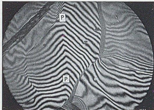
FIG. 7.—Surface Tilt at Sub-Boundary *PP* in a Fine-Grained Specimen Extended 11.9%. Interference micrograph.  $\times 310$ .
