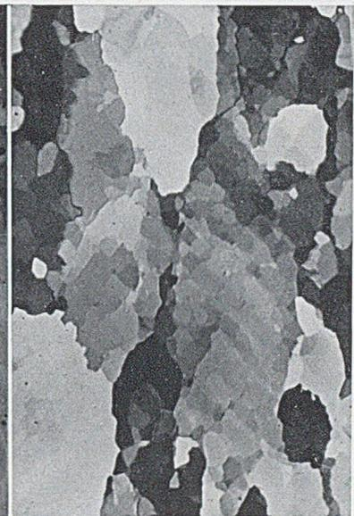
FIG. 3.—Relatively Unbanded Structure in Fine-Grained Specimen Extended 50%.  $\times 100$ .
