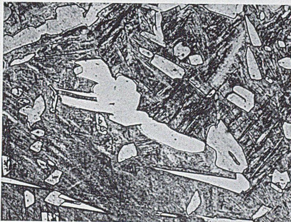
FIG. 9.—7.7 at.-% Tin Alloy (Commercial Titanium), Quenched from 950° C. Equilibrium \alpha in matrix of acicular \alpha . \times 200 .
