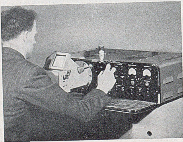
Fig. 1. Close-up view of the control desk and camera of the new Metrovick electron microscope Type EM4.
