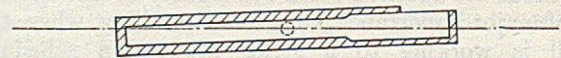
FIG. 3.—Position of Mould During the Pouring Operation by the Method Similar to the Durville System.
