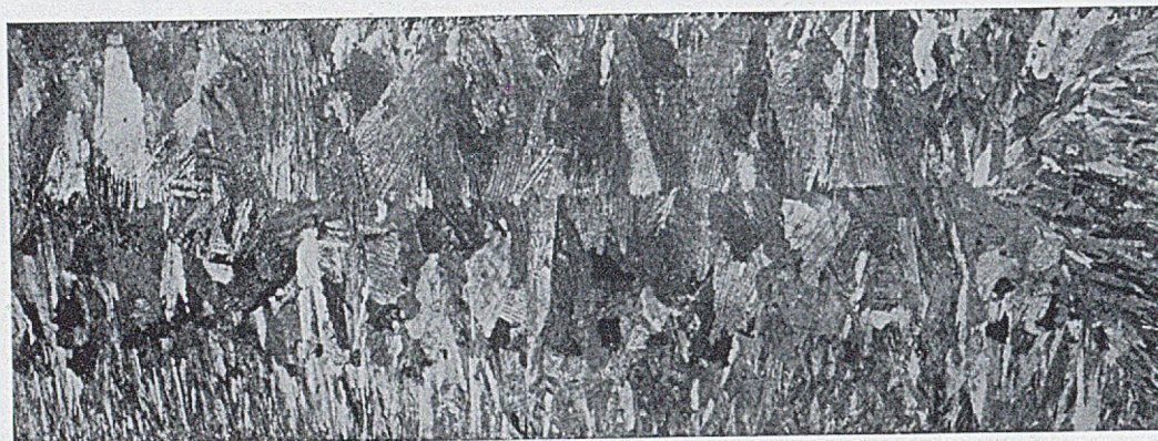
FIG. 8.—Macrostructure of Vertically Cast Zinc Rolling Slab. \times 1 approx.
