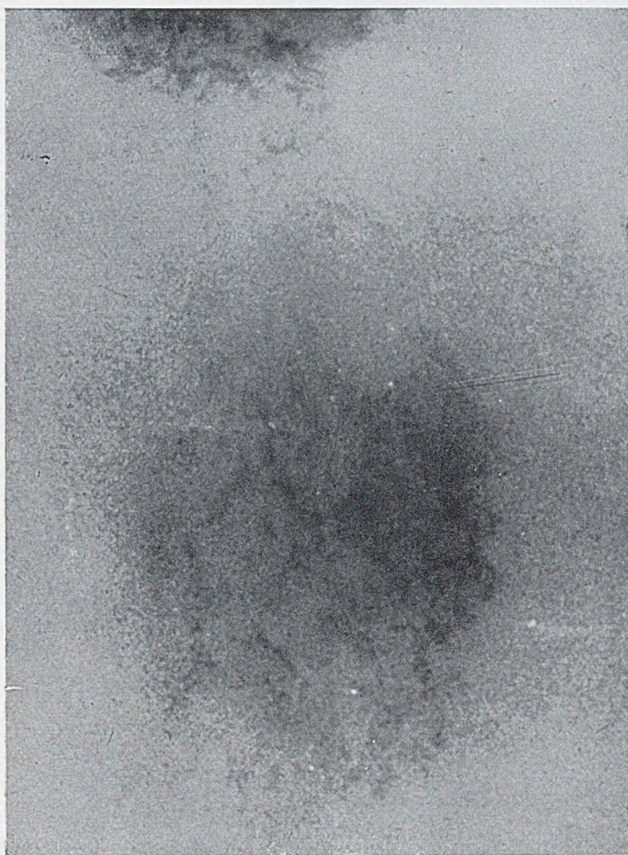
FIG. 4.—Radiograph of Zinc Rolling Slab Containing Interdendritic Shrinkage. \times 1 .
