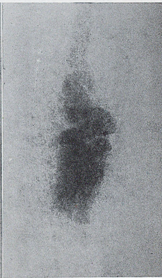
FIG. 6.—Radiograph Showing Large Gas Cavity in Zinc Rolling Slab. \times 1 .
