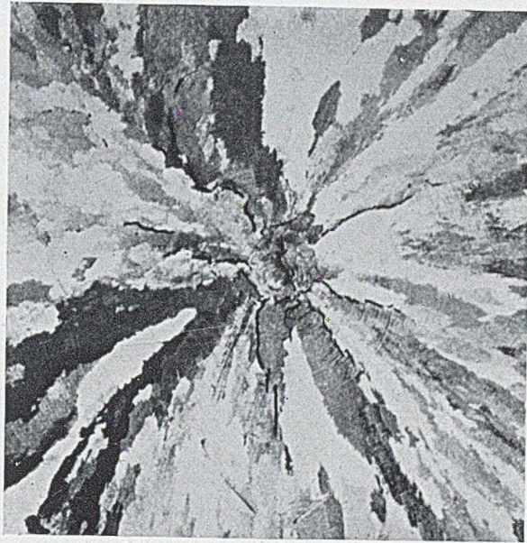
FIG. 13.—Structure at Centre of Transverse Section of 4 × 4-in. Gothic Wire Bar, in Commercially Pure Aluminium Direct-Chill-Cast. Etched. × 2.
