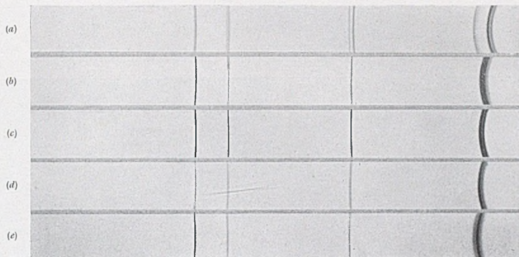
FIG. 13.—X-Ray-Diffraction Patterns of Alloys in the ( \gamma + \gamma' ) Phase Field at 750° C. (Mn K\alpha Radiation).
