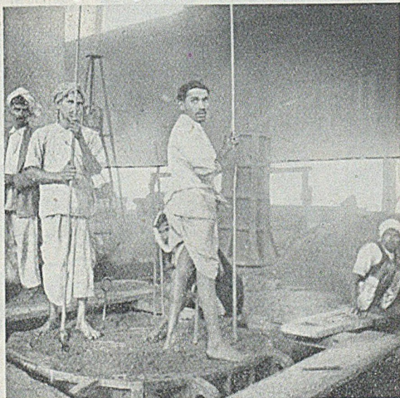
FIG. 3.—Final Ramming in Progress; a Light Core Iron is used near the Top to allow for easy contraction of the Casting.
