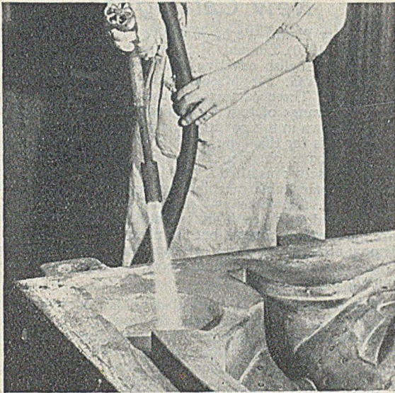
FIG. 14.—Skin Drying of a Mould by means of a Mond-gas Torch.
