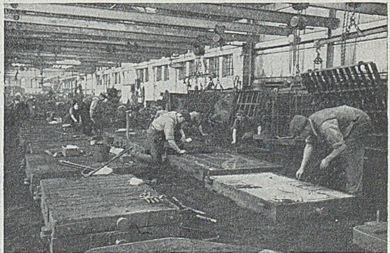
FIG. 5.—Pianoforte Frame Bay, showing Part-finished Moulds. Note the Overhead Monorail Hoists.
