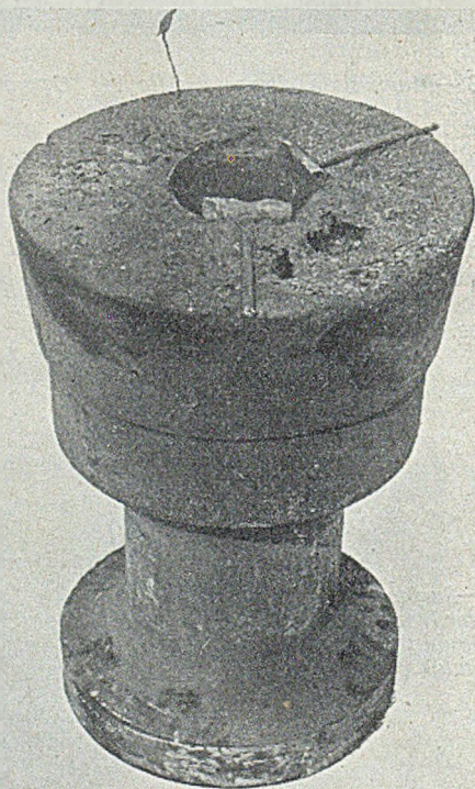
FIG. 6.—Top-poured Cylinder Casting in Spheroidal-graphite Cast Iron.
