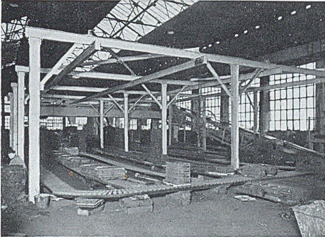
Illustration of Sand Treatment Plant in small foundry using 4 moulding machines and turning out 12/15 Tons of Small Castings per week.
