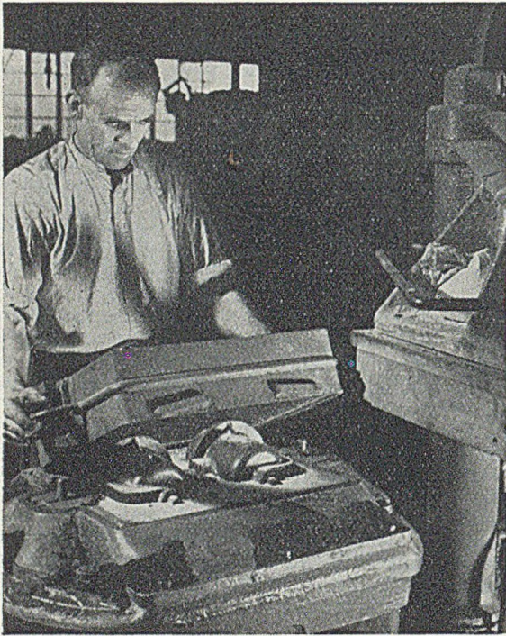
FIG. 2.—Half-mould being produced from a Jolt-squeeze Moulding Machine.
