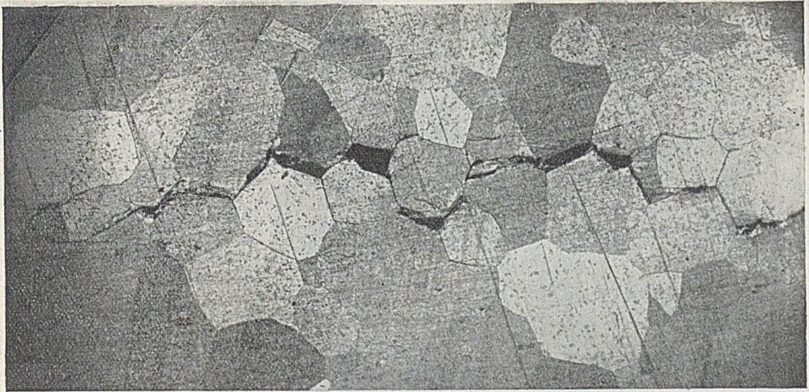
FIG. 4.—Intergranular Crack in Cast Manganese/Aluminium/Brass Coil-binding Ring. \times 25 .
