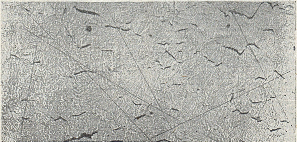
FIG. 6.—Characteristic Intergranular Cracking of a 0.5 per cent. Molybdenum Steel under Tension at High Temperatures \times 10 magnifications.
