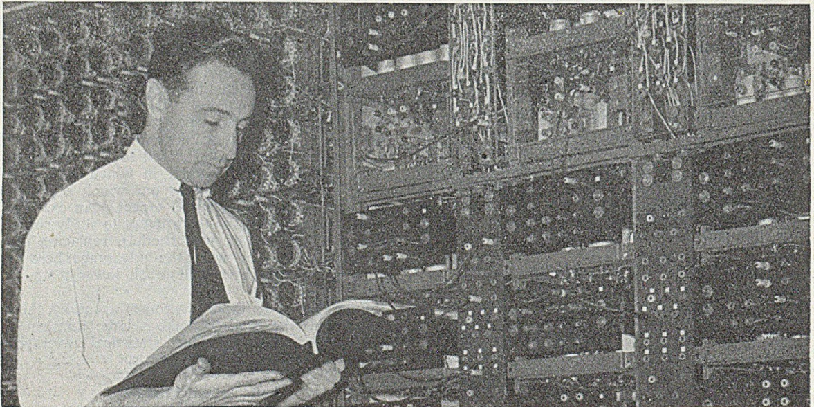
FIG. 7.—Part of the Frames with Capacitances and Resistances in the Heat and Mass Flow Analyser Laboratory, Columbia University.
