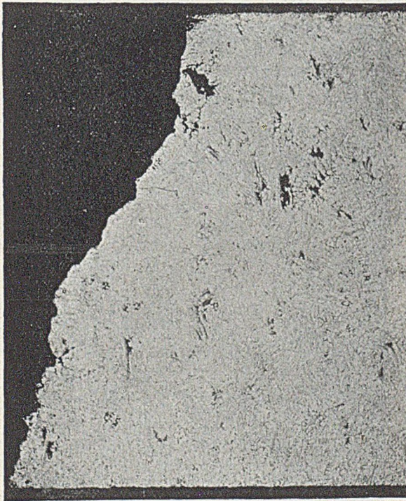
FIG. 13.—Shrinkage Porosity in LM-15 (High Silicon; D.T.D. 250). Cavities fairly well isolated but less regular in outline than in Alloys of Higher Eutectic Content. (× 6.)
