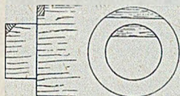
FIG. 1.—Repairs to Core-prints by the Insertion of New Pieces.
