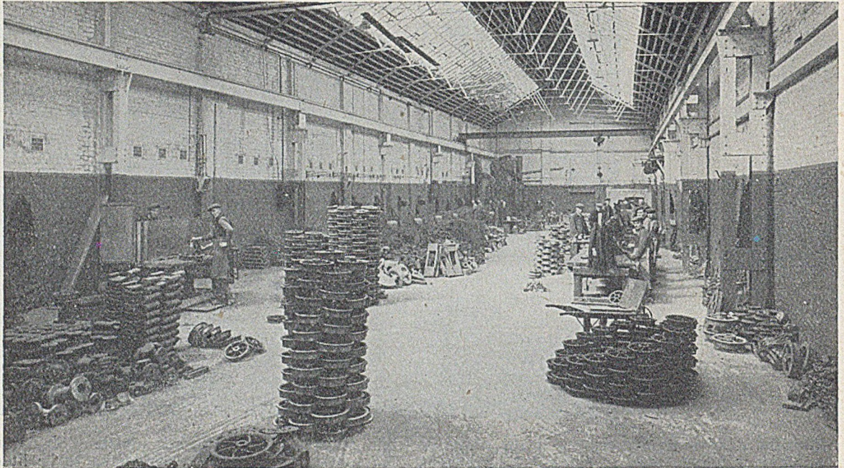
FIG. 5.—View of the Dressing Shop for Light Steel Castings. The Ample Space Available facilitates the use of Mechanical Internal Transport.
