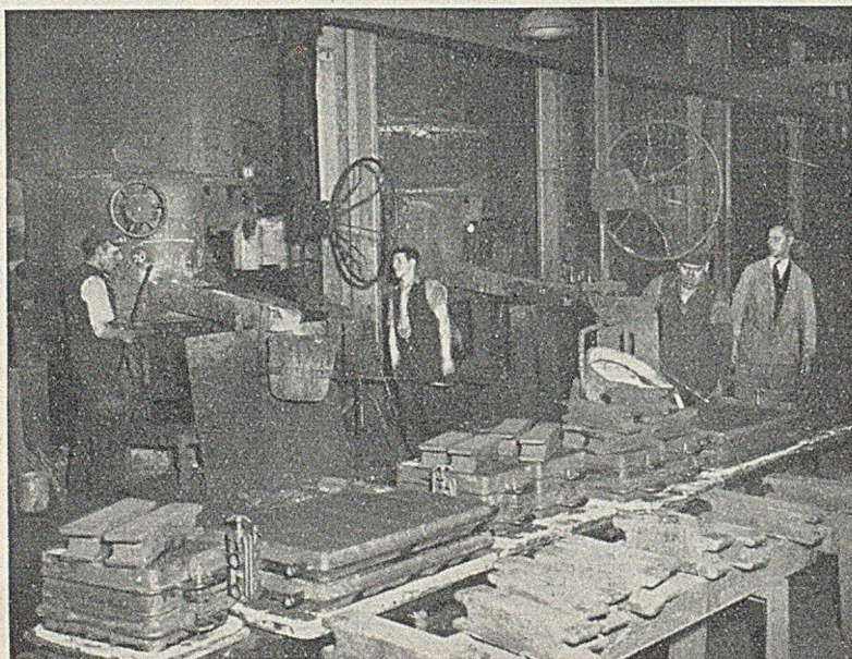
FIG. 3.—View of the Cupola Spout and Casting Conveyor with Tapping and Pouring in Progress.
