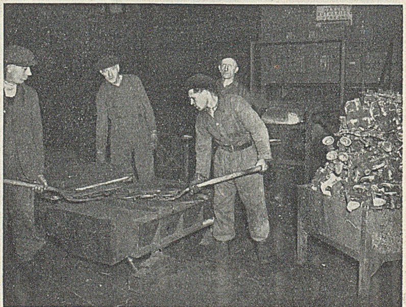
FIG. 7.—View of the Vibratory Knock-out Machine; the Absence of Fumes is Remarkable. Note the Use of a Stillage for Collecting the Castings.
