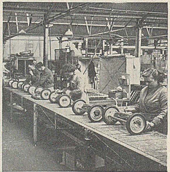
FIG. 15.—Portion of One of the Lawnmower Assembly Lines; this Production is of Rubber-tyred Machines with Cast-iron Side Members.
