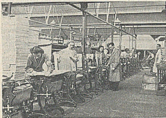
FIG. 16.—One of the Mangle Assembly Lines; the Side Members of the Machines are Left- and Right-hand Castings.
