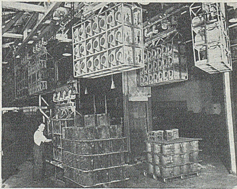
FIG. 1.—Loading and Unloading Station for the Kolene Unit. One Carrier, holding 42 Transmission Cases, is lowered to Working Level, along with a Section of Load-carrying Rail. Cases on the Pallet in the Fore-ground are Stress-relieved and ready for Loading.
