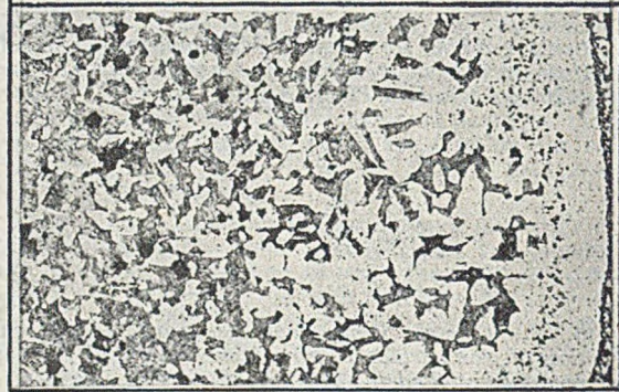
FIG. 28 (TOP).—Whiteheart Malleable. \times 200 . Etched in Picric Acid.
