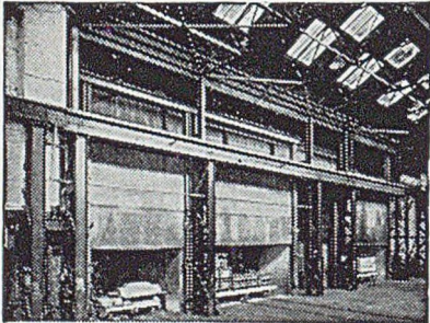
THREE N.R.S. STOVES WITH NON-WARPING DOORS AND ROLLING AXLE BOGIES
