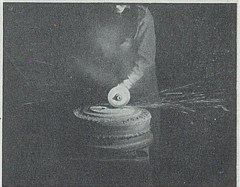
FIG. 12.—Dust Cloud from Pneumatic-drive Portable Abrasive Wheel; no Exhaust Ventilation in use.
