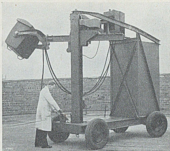
FIG. 20.—Raymax "250" X-ray Unit, shown by Newton Victor, Limited.
