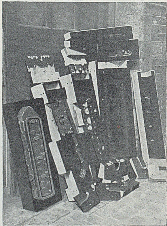
FIG. 10.—Wooden Pattern Equipment for a Motor-car Cylinder Head. This was used to produce Prototype Castings and provide Data upon which to Design Metal Production Patterns and Coreboxes.
