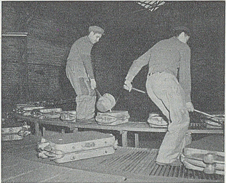
FIG. 4.—Pouring Moulds on one of the Turntable Conveyors; for this, at the present time, the Operator stands on the Grid. Magnesium-alloy Box-parts are used.
