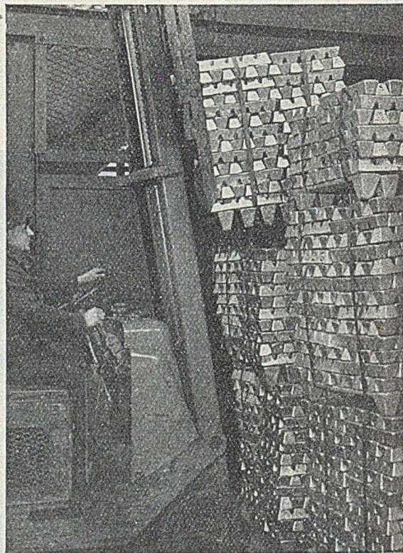
FIG. 19.—Further Illustration of Stacking Ingots; in this Case a Fork-lift Truck is being used to Stack Batches of Ingots made up as shown in Fig. 18.
