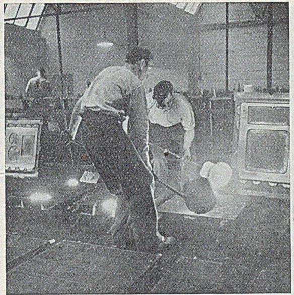
FIG. 7.—Double Pouring of Electric-cooker Castings at the Works of Belling & Company, Limited. On the left is a Pattern for a Cooker Top Plate and on the right a Pattern for a Cooker Front.
