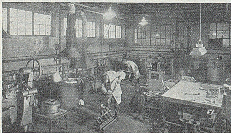
FIG. 21.—Typical Experimental Foundry where Aluminium Casting Alloys are Tested under Controlled Conditions.
